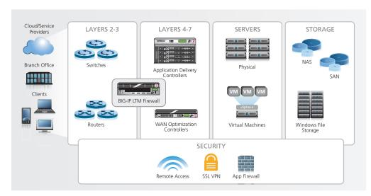
Replacing stateful firewall services with BIG-IP LTM in the data center architecture.
